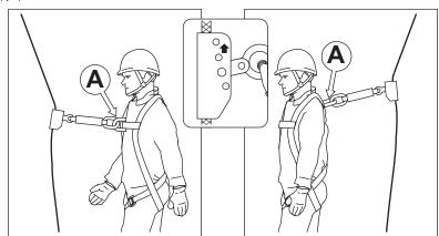
ATTENTION: Every time before using the equipment protecting against falls from height that employs the LINOSTOP II one needs to check if all the components are properly interconnected to one another and cooperate smoothly, as well as if they are compliant with compulsory standards:
